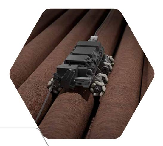
WHITEPAPER The Most Advanced Fired Heater Convection Section Cleaning Robot
